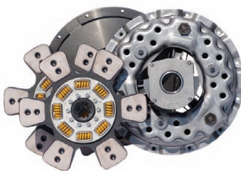
14"/352mm Single & Twin Press Steel Cover, Direct Pressure Coil Spring, Pull Type Clutch with Ceramic Driven Plate
