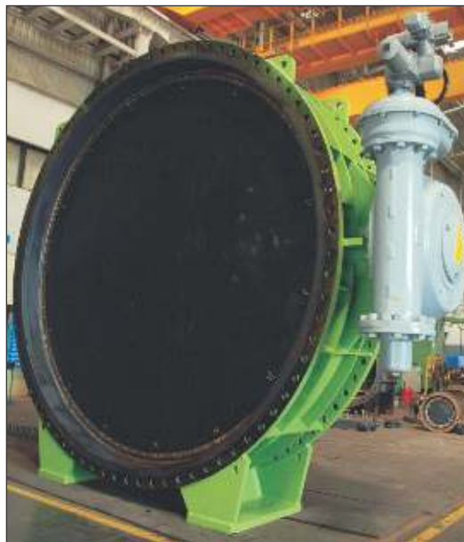
Largest size butterfly valve for thermal power plant in India. 3600 mm diameter for sea water application for 2x660 MW Essar Power Salaya Thermal Power Project
