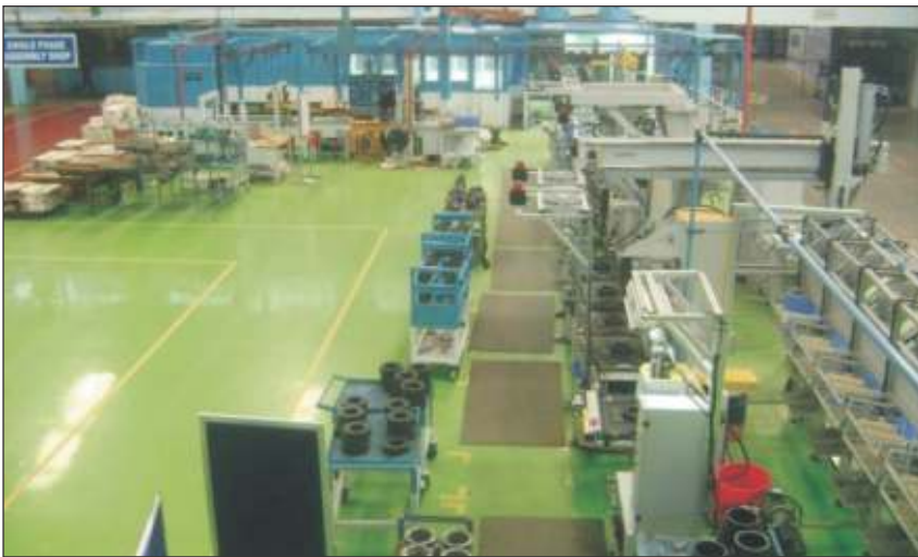
New assembly lines for single phase and KOS pumps which yielded a productivity improvement of up to 80% in Dewas.
