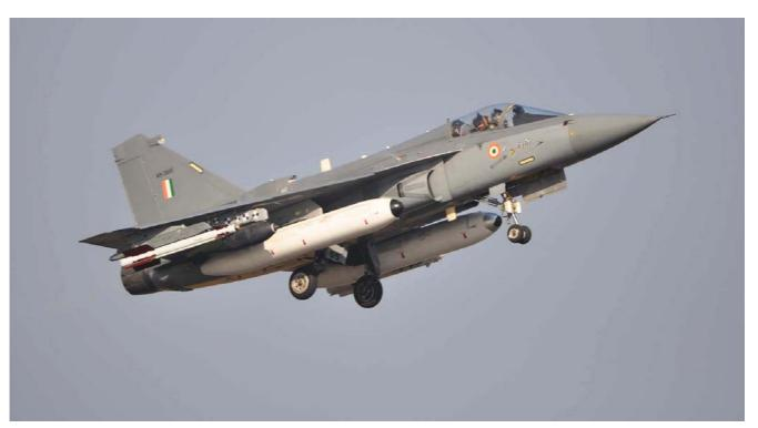
LCA with drop tanks during sea level trials
