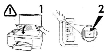
Scan this sheet to align cartridges
