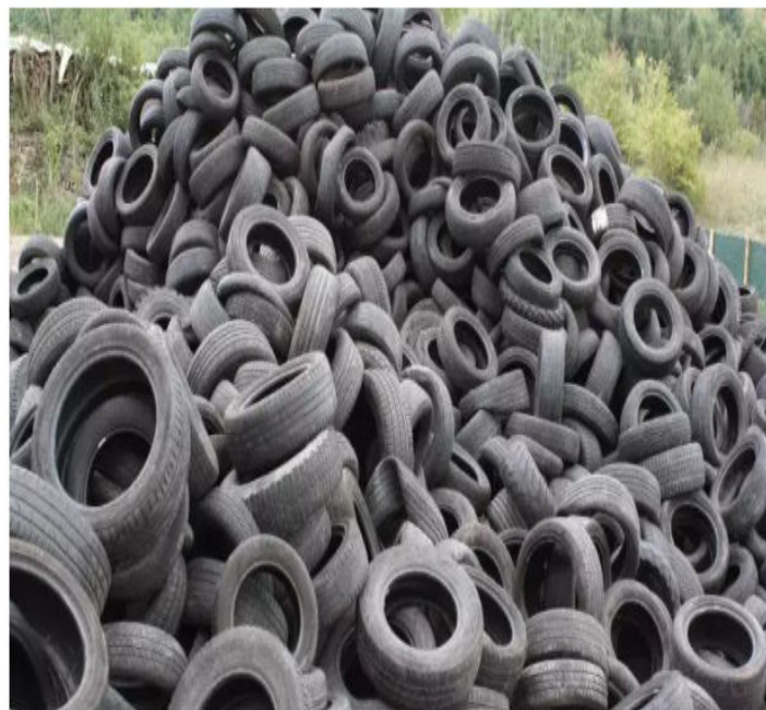
The waste tyres are recycled as reclaimed rubber, crumb rubber, crumb rubber modified bitumen (CRMB), recovered carbon black, and pyrolysis oil/char.
