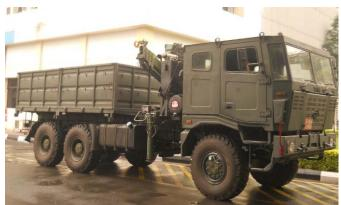
Developed indigenously, the Tata 6X6 high mobility all-terrain all-wheel drive vehicle, has completed a total trial duration of 25 months, demonstrating maximum performance in the most demanding conditions. Designed to cope with extreme on or off-road loads, these vehicle have gone through trials like waterfording, on cross country terrains and plains and at VRDE's (Vehicle Research & Development Establishment) torture track.
