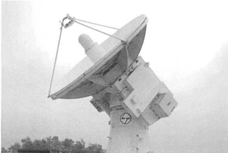
A view of the S-band Radar supplied by L&T. Photo courtesy: ISRO
