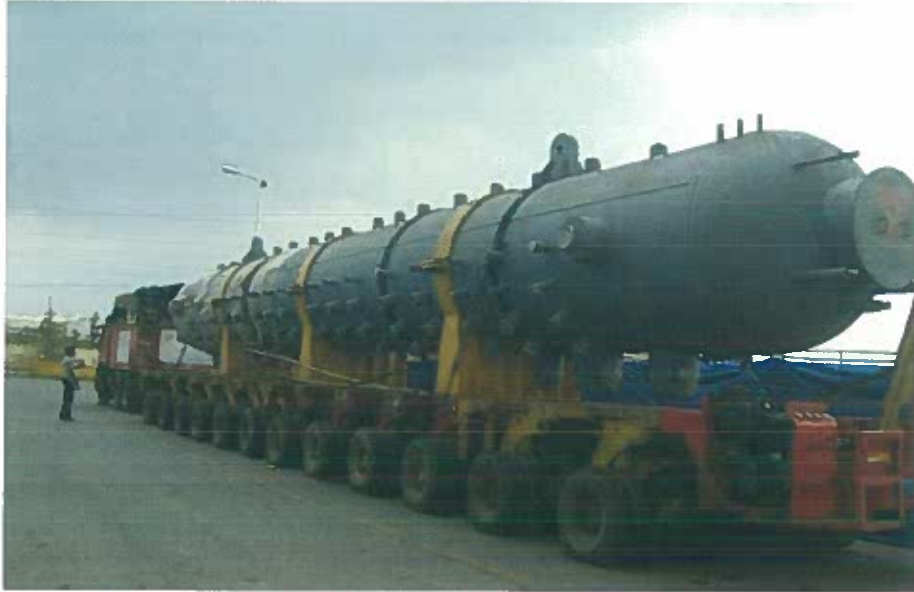
Steam Drum taken from Savil to Dahej, for the largest order won by Thermax, for a petrochemical major (Weight 157 MT)
