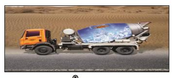
**Thermocrete** is temperature controlled concrete used for mitigating termal tensile cracks
