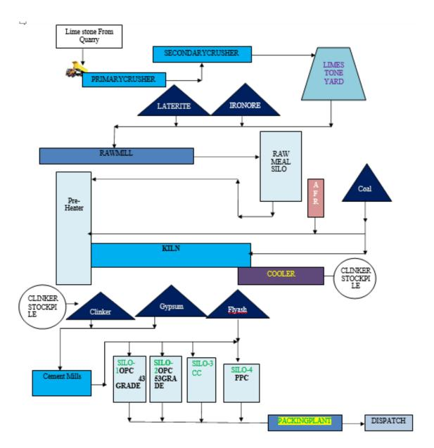
Set out below is the brief write up on the manufacturing process beginning with the manufacturing of clinker and ending with cement production. Cement is primarily a processed mixture of limestone, sand, shale, clay and iron ore, with limestone being the major rawmaterial.
