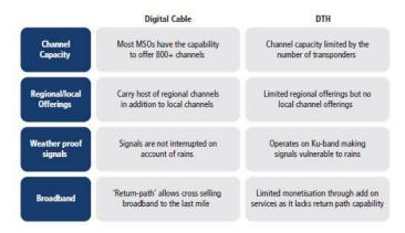
Note: 'Return-path' in the above chart refers to the upstream transmission, i.e. carrying signals from the subscriber back to the head-end. This allows a subscriber to order movies, for example, and use other additional services.
